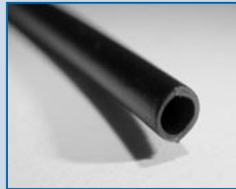
Prototype fibers and tubing for advanced thermally conductive fabrics to be used in future space suits
