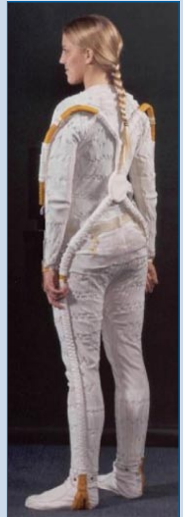
Prototype fibers and tubing for advanced thermally conductive fabrics to be used in future space suits
