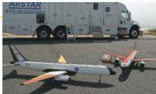
The AirSTAR flight testing facility and the Generic Transport Model developed by NASA Langley
