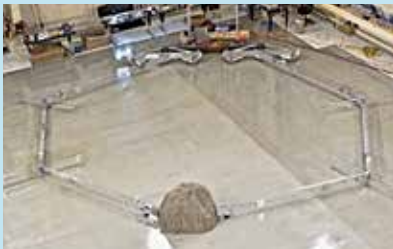
Figure 2. Prototype TALISMAN Hardware posed to grapple a free-flying asteroid.
