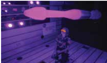
Figure 1: Illumination of PSP on a model surface at NASA Ames; photo credit NASA
