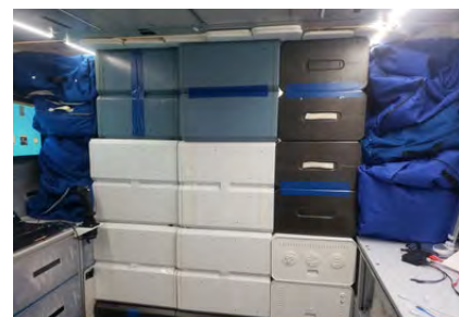
Figure 2 – A combination of CTB's and locker trays constructed to create a storm shelter wall. (Credit: NASA)
