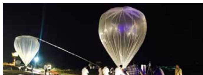
Figure 2 - Flight preparation at the balloon facility of the Tata Institute of Fundamental Research, Hyderabad, India, in July 2019. The main balloon is inflated on the left, while a secondary balloon is used near the main payload to facilitate the launch.
